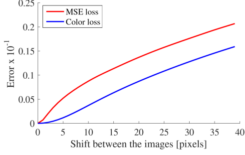
Figure 5. Comparison between responses to small image pixel-shift of MSE loss and Color loss. After applying the Gaussian filter in the original feature maps, the color loss is more pixel-invariant to the MSE loss
