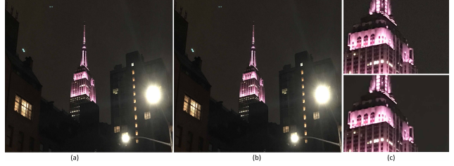
Figure 3. Side-by-side denoise comparison: (a) Denoised result using real-world data for training (training data generated by multi-frame denoising). (b) Denoised result using synthesis data for training (training data generated by adding Gaussian noise to clean images). (c) Close up comparison, where on the top is the closeup of (b), on the bottom is the closeup of (a). It can be observed that using real-world data for training leading to obvious improvement in the single sub-task of denoising, which could indicate that the potential problem of using synthesized training data.
