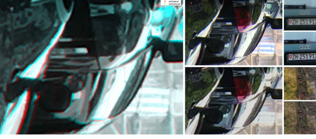
Figure 2. Difficulties in image registration due to different sensors and optics: The left image is the result of registration, in which the red and blue area indicate the imperfect alignment. It can be observed that even with camera registration, misalignment still exists, this problem is also reflected in another similar dataset[2].
